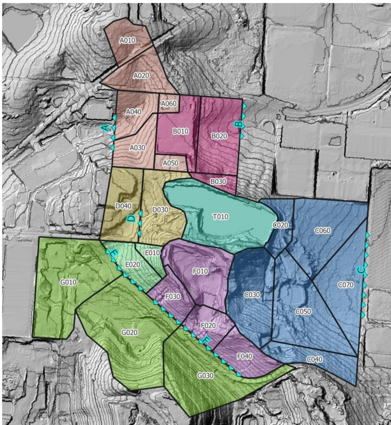
Figure 20 Existing Sub-Catchment Delineation
